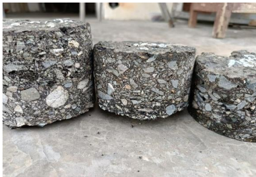
Gambar 3.5 Sampel core drill
