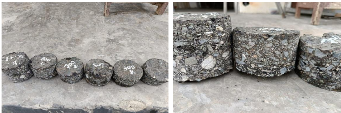
Gambar 4.2 Sampel pengujian core drill
