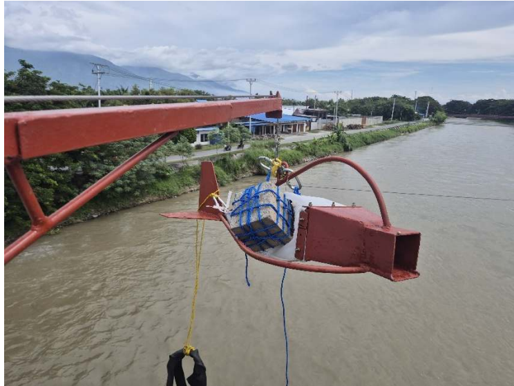
Gambar 3. 3 Alat Pengambil Sedimen Transpor Tipe Helley Smith
